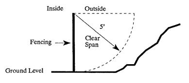
Figure <sup>31B-5</sup> Effective fencing height.
